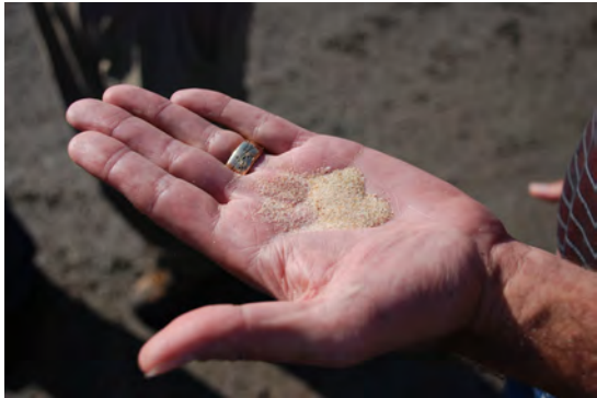
Fine-grained silica sand is mixed with chemicals and water before being pumped into rock formations to prevent the newly created artificial fractures from closing after hydraulic fracturing is completed. Photo: Bill Cunningham, U.S. Geological Survey
